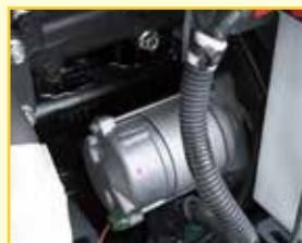
Starter motor Generator
