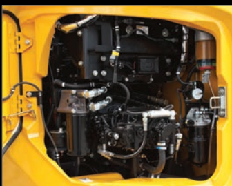
Fuel filter / Fuel filter with build-in water-separator
