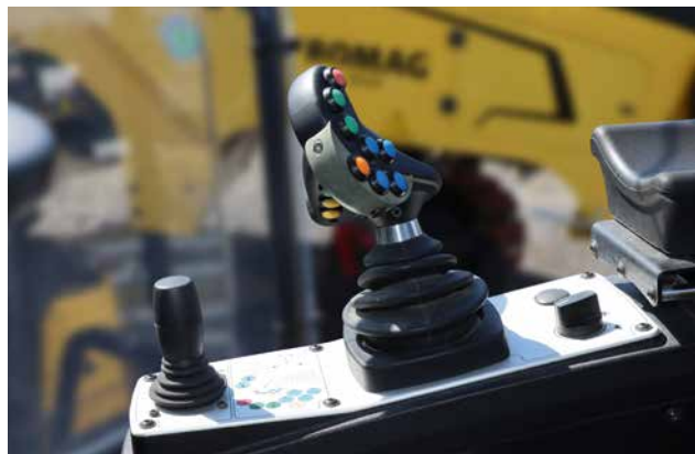
All in the operator's hand: multifunctional travel lever.
