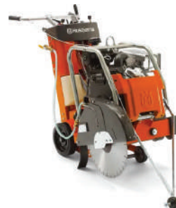
18 inch self Propelled Walk Saw
